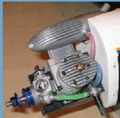
The Evolution .36s are slightly angled on the firewall to minimize their impact on the silhouette while airborne, and still keep the
