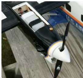
The nacelles each have a large hatch with a simple spring loaded catch. Designed for battery changes for electric fliers, it is also a great aid for accessing the fuel tanks and matching fill levels before flight.
