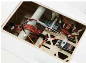
The large access hatch allows you to easily connect the aileron, flap and throttle servo leads while assembling the otter at the field.
