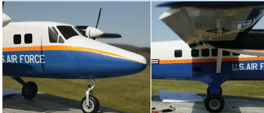
The oleo nose gear strut goes a long way to smoothing out a rough field, and looks fantastic as you taxi back after a flight. The slotted flaps are very close to scale in operation and provide a noticeable benefit when both taking off and landing.
