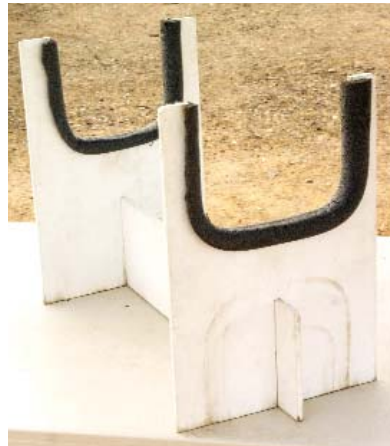
8 Quarter-inch plywood, cushioned with rubber pipe insulation was used to make this quick stand. The cutouts for the fuselage can be made to fit any model exactly.
