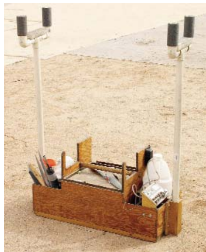
10 A great stand for modelers with aching backs. Pipe holders were attached to the ends of the flight box. PVC pipes, with cushioned fuselage holders, were cut to the modeler's height and inserted into the pipe holders. They can be removed for transportation.
