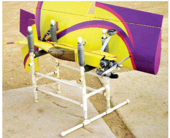
6 Ollie Edwards added outriggers to his stand to hold the wing for transportation. Note the pipes added to the bottom of the frame to add lateral stability.
