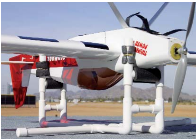
4 Your stand should be high enough to keep the propeller and fin/rudder off the surface when the fuselage is inverted, and the wheels shouldn't touch the surface when the plane is upright.
