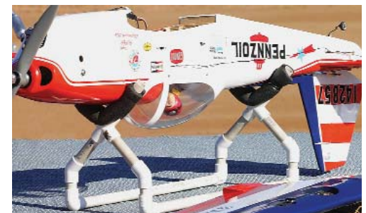
12 A nice construction but it's unstable. The bottoms of the curved fuselage holders do not match the fuselage's flat bottom. ☹️
