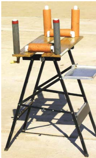
7 A unique plane holder made using an adjustable bench that's available from the tool section of most chainstores and department stores. The PVC frame fits into holes drilled in the bench's wooden platform.
