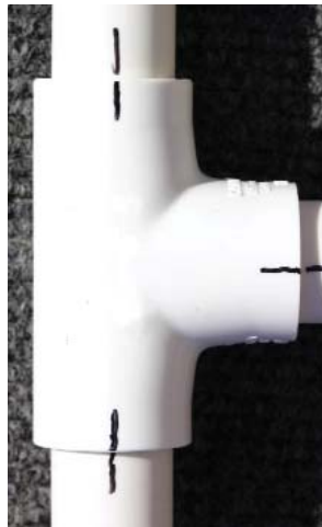
5 When the completed frame is adjusted and sits flat, mark every joint like this.
