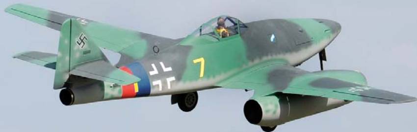
Joe Saitto's Me 262 is scratch-built, powered by a JetCat P-120 and weighs 36 pounds.
