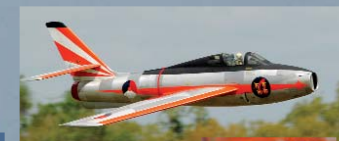
Brian O'Meara's F-84G is from a "Phantasy in Blue" kit out of Holland. It is powered by a Jet Cat 200 turbine and equipped with a smoke system. It won MAN's Best Military Award.
