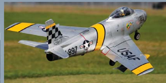
Jack Diaz owns this beautiful F-86 Sabrejet, which was built in 2005 from a BVM kit. It is 1/4 scale with an 80-inch span and is powered by a Jet Cat P-160 turbine. The model is built with operational speed brakes, landing and navigation lights, Fowler flaps, sliding canopy and droppable external fuel tanks. Since its completion in 2005, it has won several awards at Top Gun and many Best Craftsmanship awards at various events.
