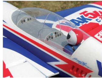
The pilot figure, cockpit and canopy are pre-installed, which saves building time. Note the five angled vent-holes behind the pilot.
