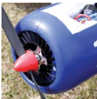
The Yak's motor mount was replaced by one from "small parts CNC"; it is machined out of aluminum stock and fits perfectly.
