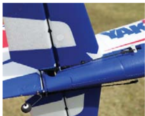
There are a few plastic parts throughout the airframe, which add even more strength to areas that could easily get damaged. Note the bottom of the tail cone and the rudder. You can also see how the stabilizer is held in by a screw (one per side) and that the rudder's carbon fiber pushrod is longer than the elevator's. The tailwheel comes pre-mounted to the rudder.
