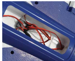
The radio compartment is covered with a plastic, tab-fitted hatch that is secured with a screw at the aft end. Its receptacle is also made from plastic.
