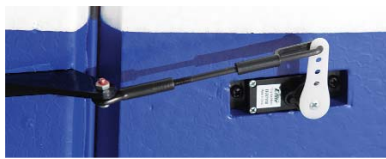
The aileron servos, pushrods and control horns are all pre-installed and ready to go.
